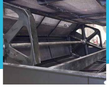
REBUILT SCREENS ARE FULLY DISASSEMBLED, BLASTED TO BARE METAL, AND REASSEMBLED WITH NEW WEAR COMPONENTS, READY FOR EXTENDED SERVICE AT YOUR INTAKE.
